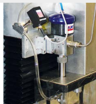
Control System Backflow interrupts the high pressure jet if the abrasive gets stuck when incoming to the cutting head.
