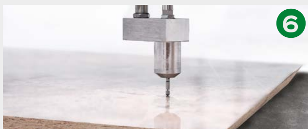
Electronic feeler for automatic measuring of the thickness of the slab to cut indispensable for a perfect cutting at 45°.
