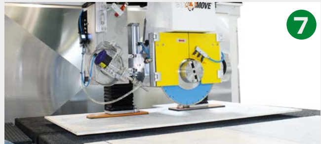
Manipulator with suction cups for the automatic movement of the work-pieces. Prussiani Engineering European Patent EP 1651409. Manipolatore a ventose per lo spostamento automatico pezzi. Brevetto Europeo Prussiani Engineering EP 1651409.
