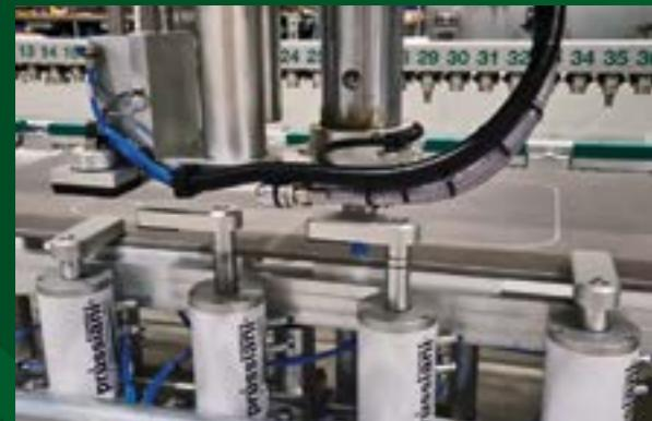
**PNEUMATIC TONGS** The clamping of the workpiece is ensured by suction cups and pneumatic tongs, also available in a rotary version, which automatically rotate to allow the tool to pass through, then they return to position and restore the clamping.
